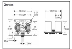
Fig 2: Dimensions of Ultrasonic Sensor
