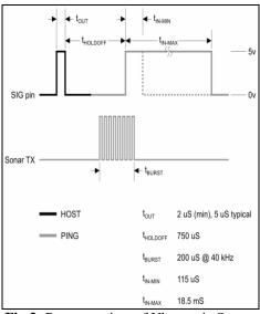
Fig 3: Response time of Ultrasonic Sensor
